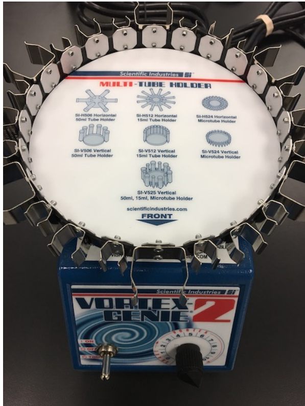
Figure B-1: A Vortex Genie 2 vortex mixer fitted with a vertical 50 mL tube holder with a 6 50 mL tube capacity.
