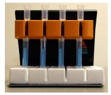
QuadroMACS<sup>™</sup> Separator with LS Columns. Elution tubes placed directly underneath.
